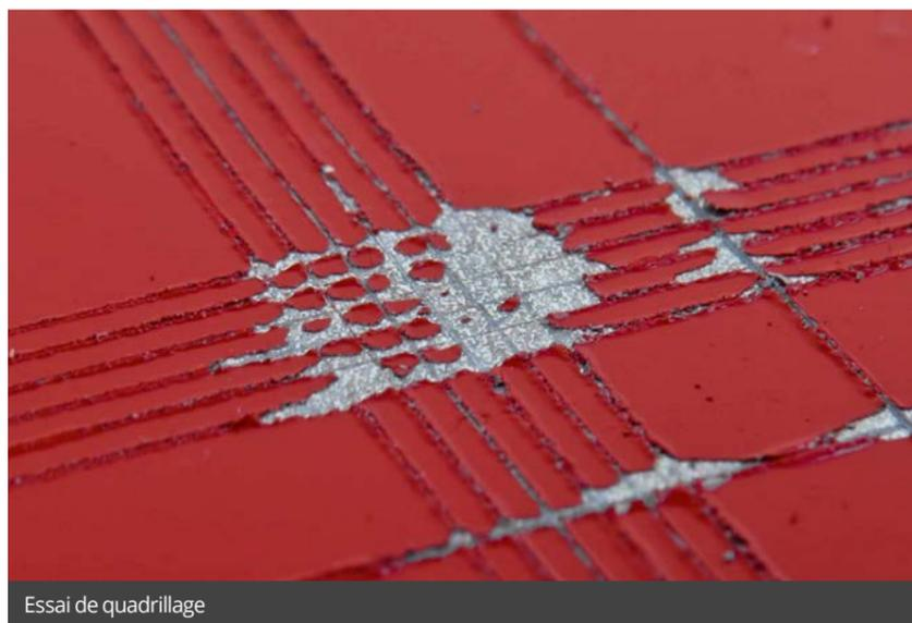
Essai de quadrillage
